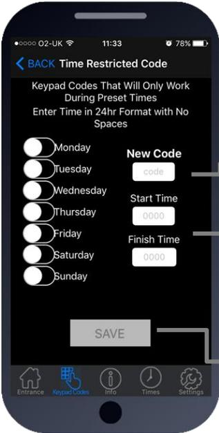
Up to 20 codes can be added which will only operate during pre-set times and days of the week. This is useful to improve security by giving pin codes which will only work during desired hours and days of the week.
