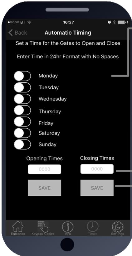
STEP 1 – Select days and an OPENING time, and press Save button below. Send the SMS to program the desired opening time.
