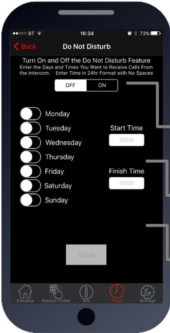
Quick turn ON or OFF. Note: turning ON without any times being entered will disable the call button all of the time!
