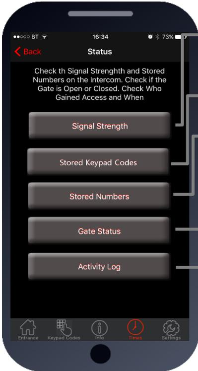
Can be used to check if the intercom reception is ok. You will receive a SMS reply with a signal level on a scale of 1-31
